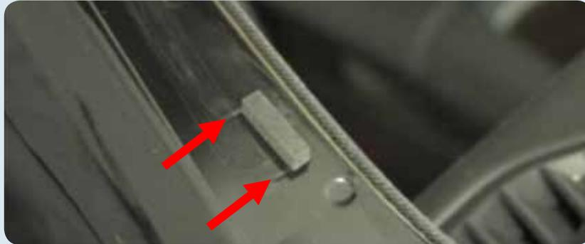
Note: It is important to place the spacers exactly between the corresponding markings on the body (see above).
