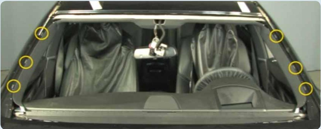
Three windscreen spacers are located on the left and on the right A-pillar as shown.
