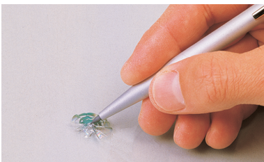
1. The impact spot is cleared of dirt and loose glass fragments, ...
