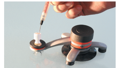
3. the injection cylinder is screwed in and filled with roger's filling resin, ...
